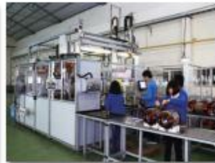
IE3全自動馬達繞線/ 入線/整形機與生產線 IE3 Automatic motor Stator winding/ Wedge Inserter/ Coil Forming Machinery and Production Line
